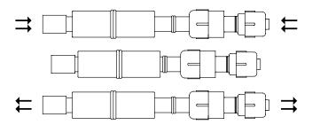
IMPORTANT For use on: Polyethylene and PVC gas pipe meeting ASTM D 2513
